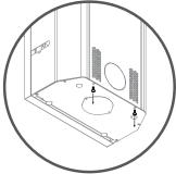
Undo all screws fixing top cover and loosen two bolts fixing the rear cover to the base. Remove the top cover of the furnace.
