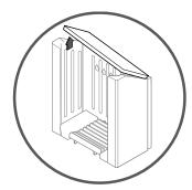
Lift one side of deflector and then lift the whole deflector upwards in such a position. Slide it slightly to the left or right to place it in free space between the side panels.
