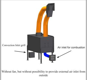
If no possibility to have external air inlet from outside or from a shelter, you can install the appliance. But ! You have to connect the air inlet 100 mm with a tube to a grill in the masonry. In this way you will provide the Venus Green Plus with Oxygen coming in from the living room. Please keep this livingroom adequately ventilated to avoid under pressure. This type of installation is not advised for Passive houses. (As same for installation with fan in this way)
